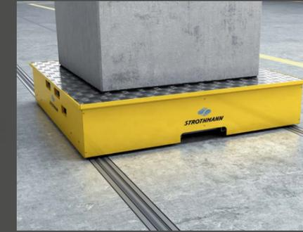
Height tolerance  $\pm 1$  mm over a 5 m track, tolerance of the track gauge,  $\pm 0.5$  mm
