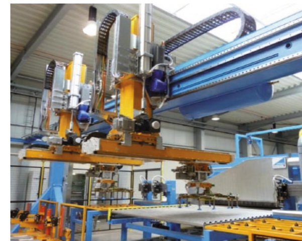
Blank destacking with double feeders and 4 blank carriages
