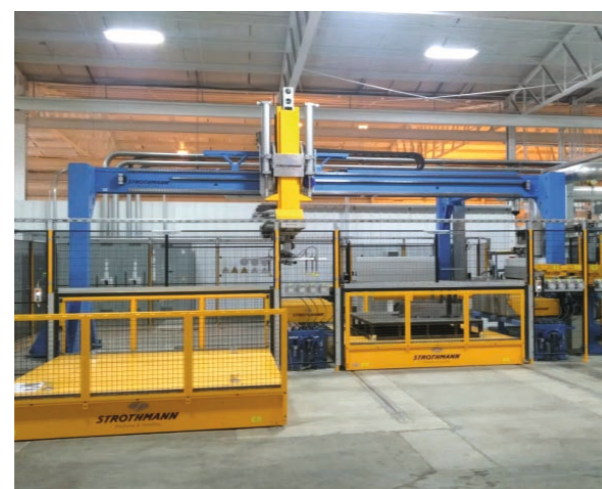
Blank destacking with magnetic spreading station
