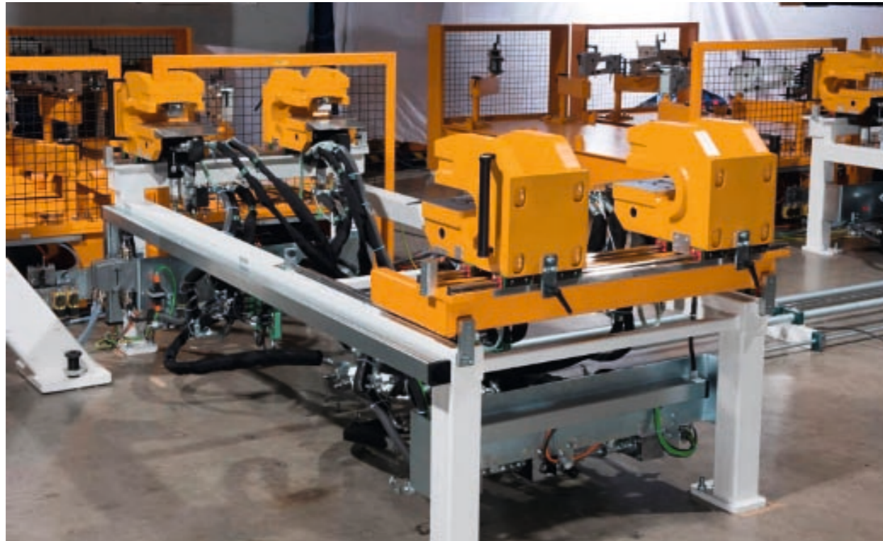
Hydraulic marking station with 2 heads arranged on opposite sides, lengthwise and crosswise
