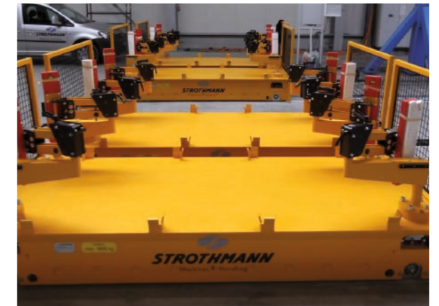
Blank destacking using pantograph arms mounted on the blank carts.
