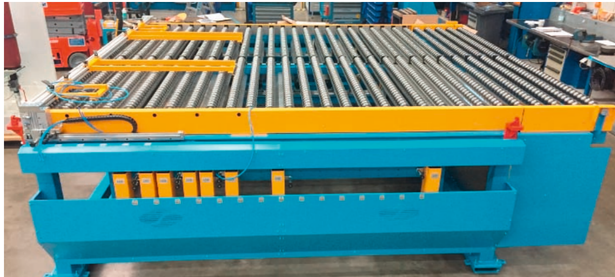
Flexible, modular centring station with servo-controlled centring fingers
