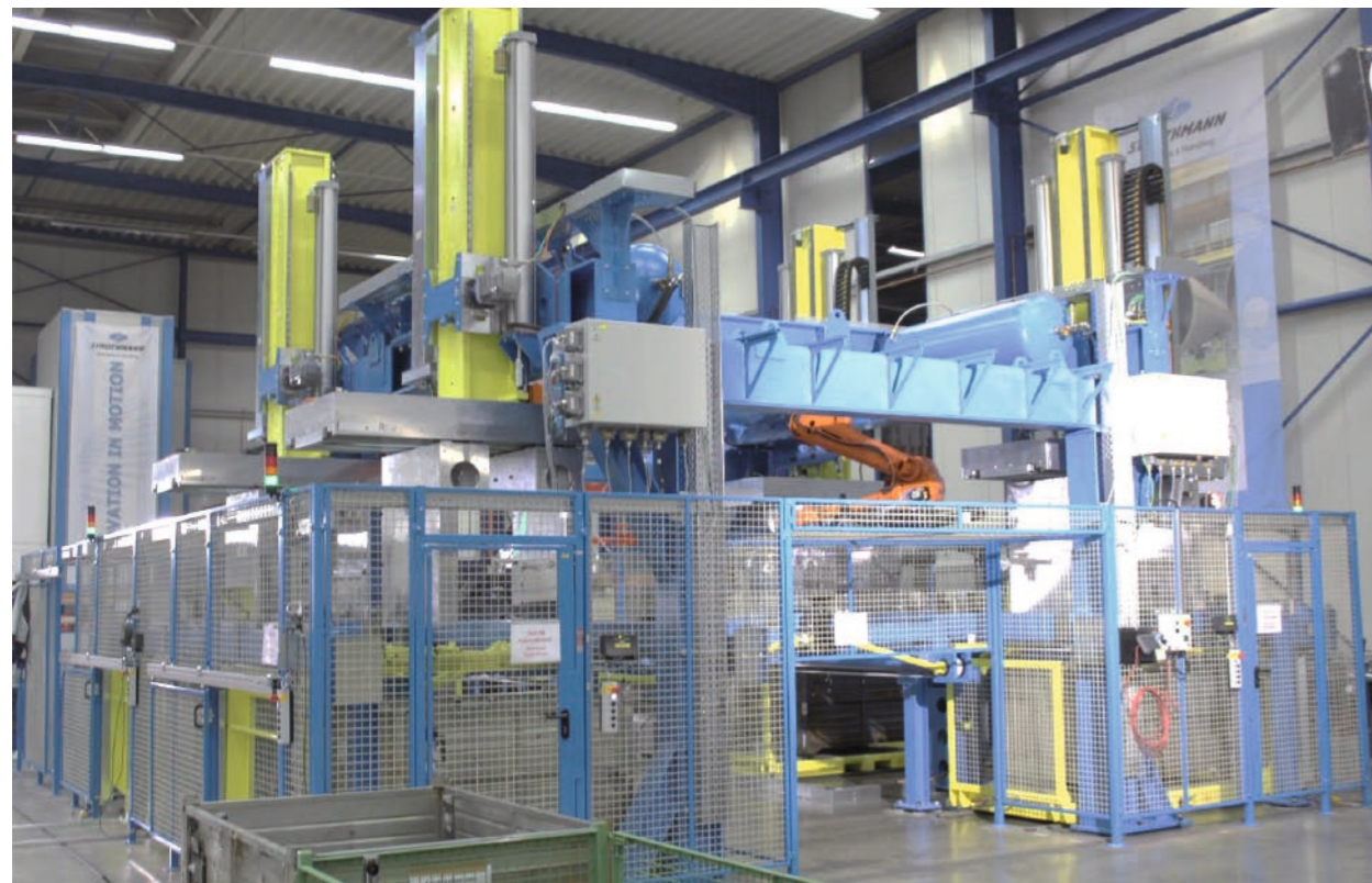
Example of automatic finished part destacking for 4-piece batch
